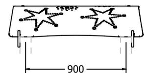
Fixing holes for roof to posts to be drilled on site
