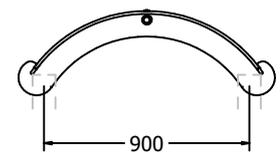
Designed to fit post centres between 900mm<sup>2</sup>
