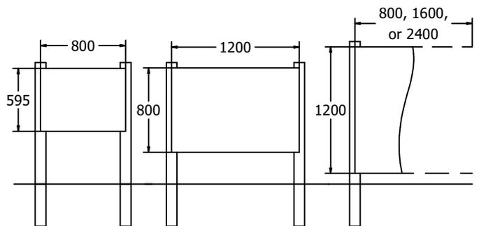
Designed to work with Fahr standard panel sizes
